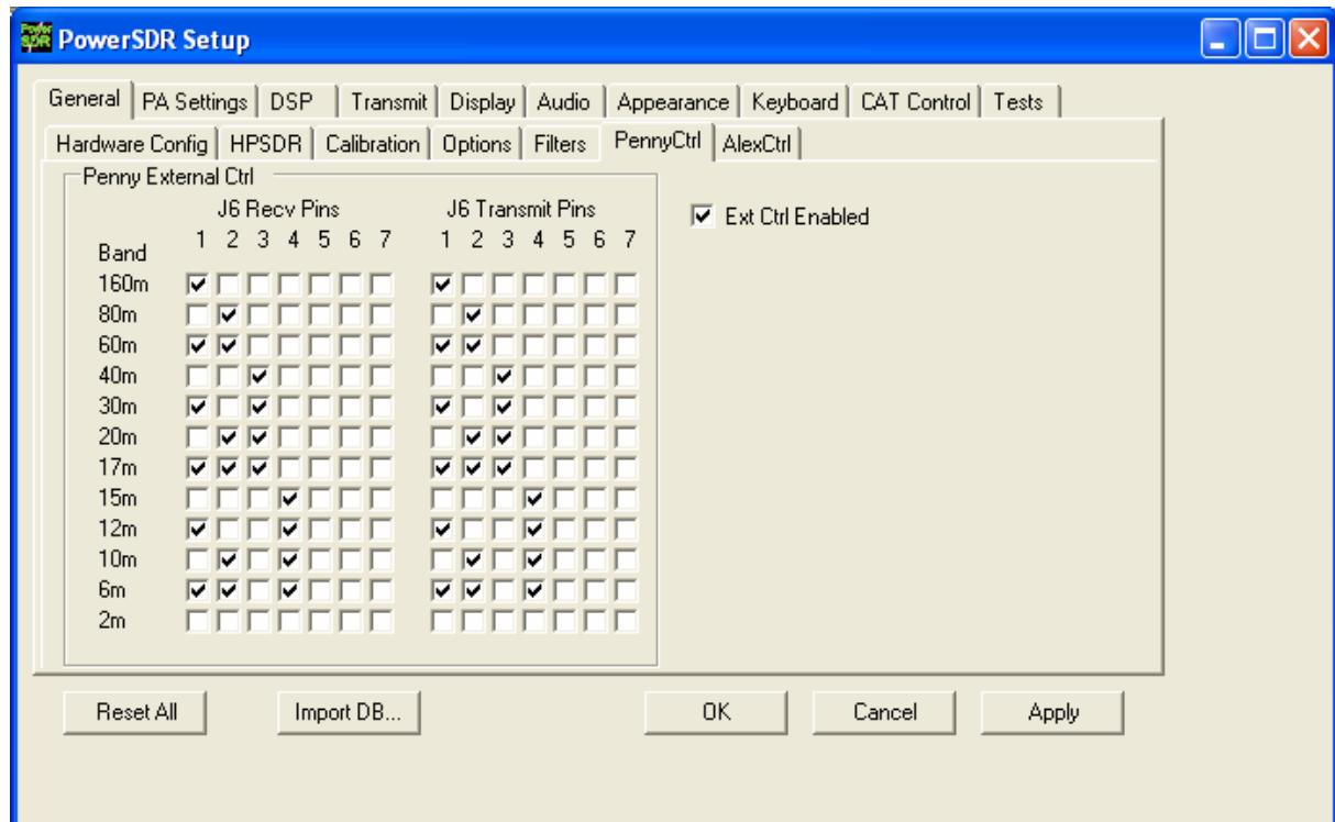
Outside the amateur bands the 6m LPF is always engaged. This makes it possible to receive frequencies outside the amateur bands without attenuation through the LPF.
