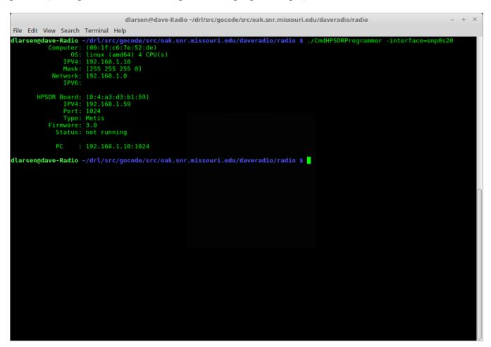
Figures 4 is the output of the Protocol 1 command line programmer after discovery of a Metis board.
