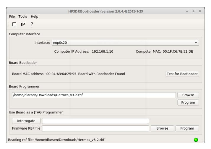
Figure 2 is a diagram of the HPSDRBootloader program after Board discovery and prepared to program the Hermes board..
