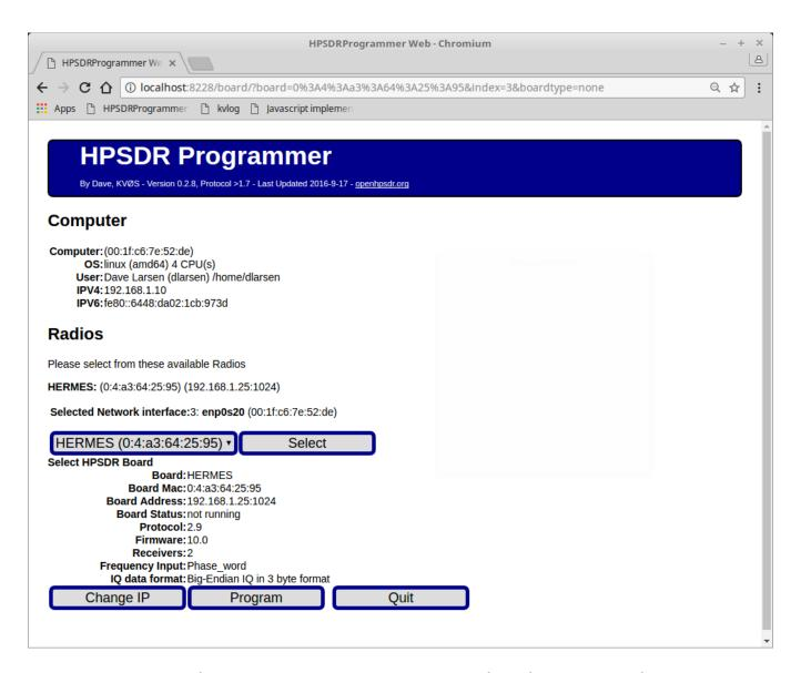
Figure 6 is a Diagram of how the HPSDRProgrammer web interface after discovery of a Hermes board.
