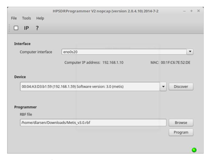
Figure 3 is a example of the HPSDRProgrammer\_V2 program with the metis board discovered and ready to load the firmware into the board.
