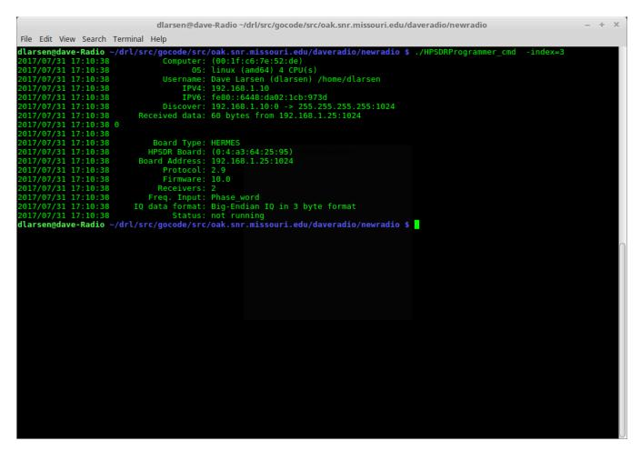
Figures 5 is the output of the Protocol 2 command line programmer after discovery of a Hermes board.
