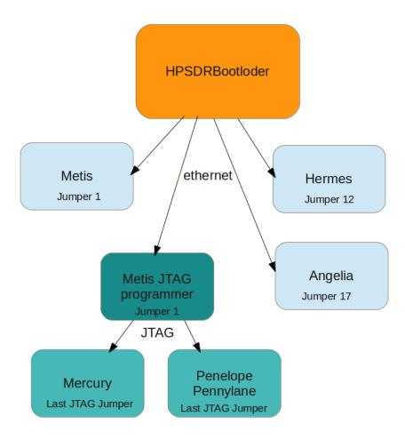
Figure 1 is a diagram of how the HPSDRBootloader access the component boards of the HPSDR system.
